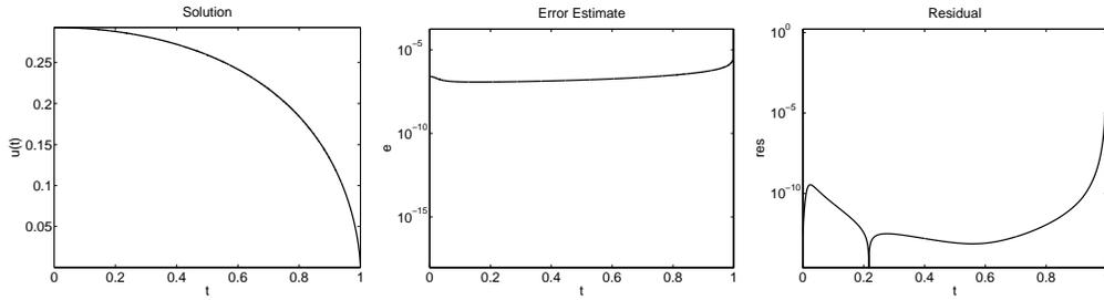
Figure 7: Problem (4.24),  $A = 0$ ,  $\gamma = 2$ : The numerical approximation for the solution component  $u(t)$ , the error estimate and the residual
