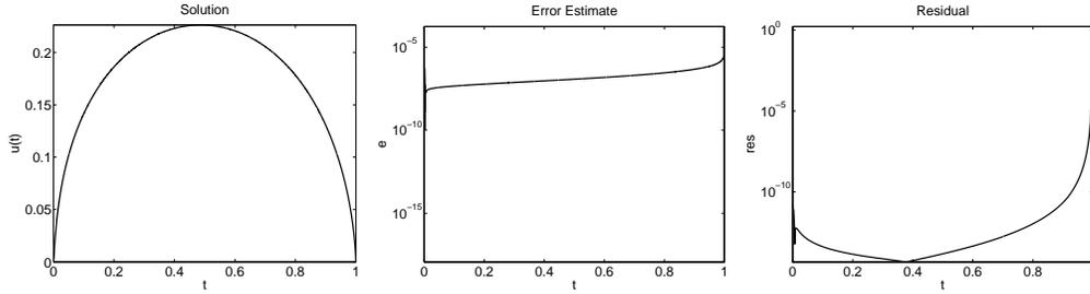
Figure 10: Problem (4.24),  $A = 0$ ,  $\gamma = 1.2$ : The numerical approximation for the solution component  $u(t)$ , the error estimate and the residual
