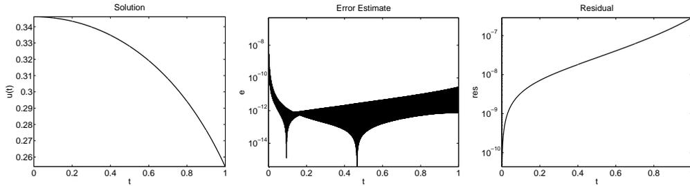
Figure 12: Problem (4.24),  $A = 0$ ,  $a_1 > 0$ ,  $\gamma = 2$ : The numerical approximation for the solution component  $u(t)$ , the error estimate and the residual
