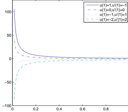
Figure 3: Illustrating Theorem 3.5 for  $a \in (-\infty, -1)$ : Solutions of differential equation (3.20) with  $a = -2$  subject to boundary conditions  $u(1) = \alpha$ ,  $u'(1) = \beta$ . See graph legend for the values of  $\alpha$  and  $\beta$ . Here,  $\lim_{t \rightarrow 0^+} u(t) = \pm\infty$  and  $\lim_{t \rightarrow 0^+} u'(t) = \mp\infty$ , or  $u(0) \in \mathbb{R}$ ,  $u'(0) = 0$ .
